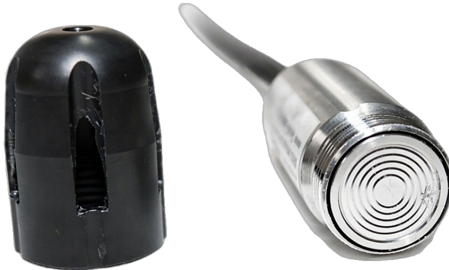
Figure 3: Piezo pressure sensor type 0312 — laser-welded stainless steel measuring cell with removable sensor cage. The oil-filled AISI 316Ti pressure cell is visible after removing the cage.
